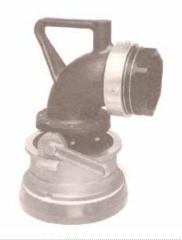
The Meggitt F250 hydrant coupler is designed to connect to 4-inch hydrants and adaptors manufactured in accordance to API bulletin 1584. Optional outlet configurations allow the use of various types of threads and hose sizes. (Supersedes F203, F230, F240 series hydrant couplers.)
