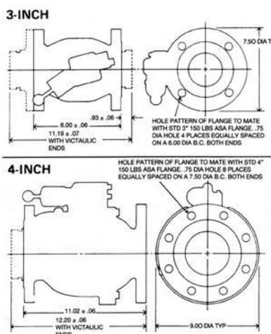
Meggitt manufactures 3-inch and 4-inch bottom loading shutoff valves for use with either the jet level sensor or float pilot valves. Refer to pages 602 and 613 for complete details on pilot controls. Both sized valves are available with ASA 150 pound flanges or ends to mate Victaulic couplings and are made of aluminum. Both valves are also available in Ductliron.
