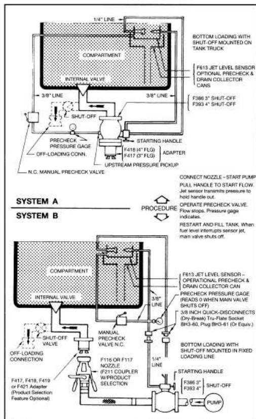
Note: F619 Float Pilot can be substituted for F613
